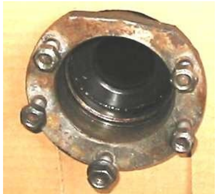
With the 65 rear axle housing apart you can see that the mounting flange is flat on top with the bolts around the remaining flange area. The 60 housing flange is completely round with the bolt pattern placed accordingly. Note on next page the backing plate shape is flat on top also to fit the flange.
