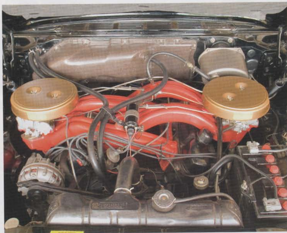
Can you imagine covering this with a plastic shroud? Ram tubes are one factor in extraordinary high-end performance; 413-cu. in. V-8 revs freely, doesn't act like a big-block
