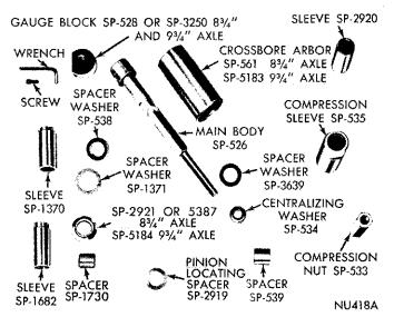
Fig. 24—Rear Axle Setting Gauge Tool C-758-D4
