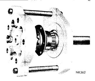
Fig. 13–Installing New Bearing and Collar
