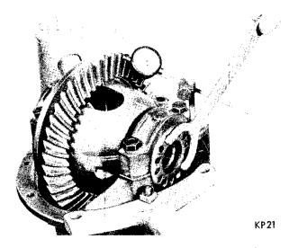
Fig. 31—Measuring Backlash between Drive Gear and Pinion
