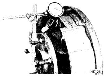
Fig. 15-Measuring Axle Shaft End Play
