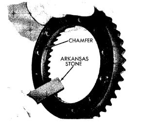
Fig. 23—Stoning Chamfer on Ring Gear
