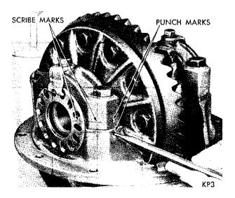
Fig. 18–Marking Bearing Caps and Adjusters
