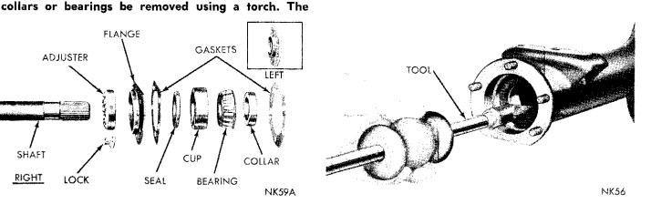
Fig. 4–Removing Axle Shaft Oil Seal
