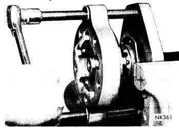
Fig. 12—Removing Bearing Cone with Tool C-3971
