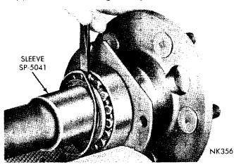
Fig. 7-Removing Roller Retainer
