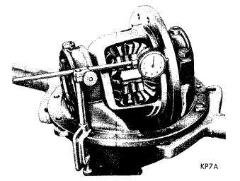
Fig. 20—Checking Drive Gear Mounting Flange Face Runout
