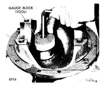
Fig. 27—Installing Gauge Block on Tool
