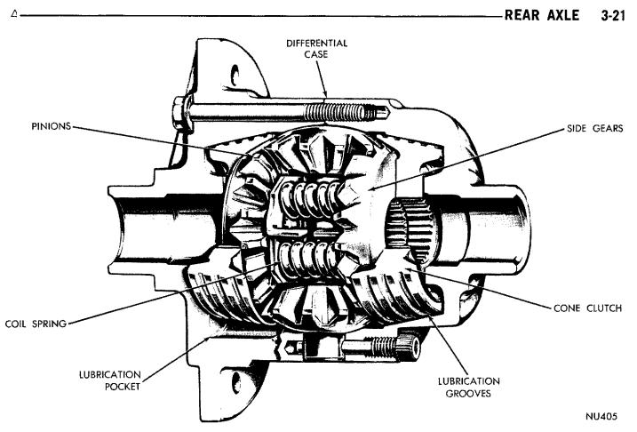
Fig. 2—Sure-Grip Differential (Schematic)
