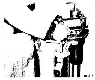
Fig. 29-Determining Spacer Thickness
