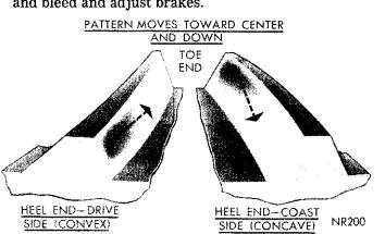
Fig. 34—Effect on Tooth Contact Pattern as Spacer Thickness is Increased
