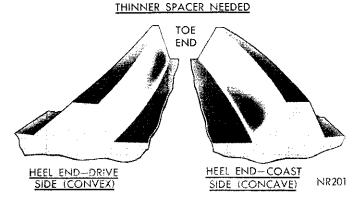
Fig. 35—Incorrect Tooth Contact Pattern (Decrease Spacer Thickness)
