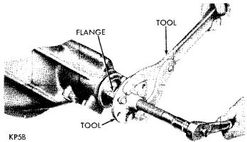
Fig. 17-Removing Companion Flange
