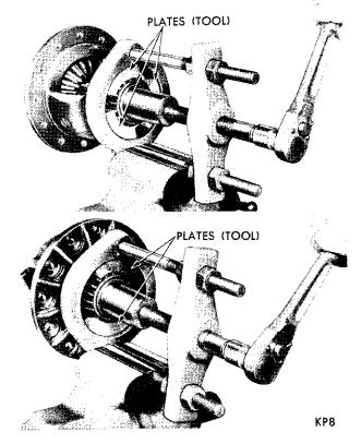
Fig. 22—Removing Differential Bearings
