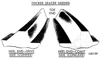
Fig. 33—Incorrect Tooth Contact Pattern (Increase Spacer Thickness)
