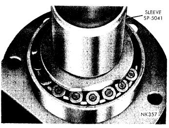
Fig. 8-Flange Ground Off Inner Cone
