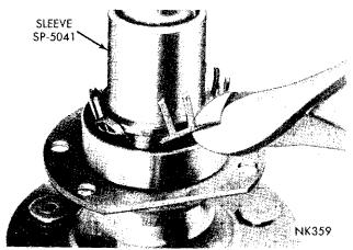
Fig. 10-Cutting Out Roller Bearing Retainer
