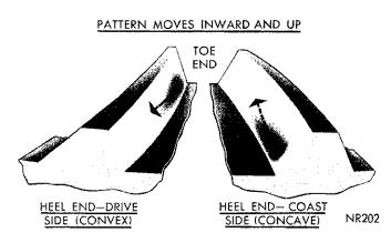
Fig. 36—Effect on Tooth Contact Pattern as Spacer Thickness is Decreased
