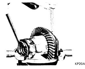
Fig. 30-Adjusting Differential Bearings
