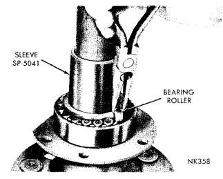
Fig. 9-Removing Bearing Rollers
