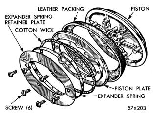
Fig. 26 — Disassembly of Vacuum Piston
