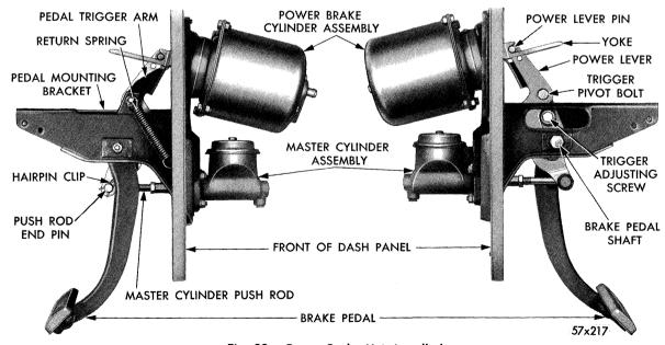
Fig. 28 — Power Brake Unit Installed
