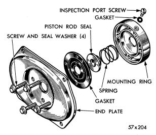
Fig. 27 — Removal of Mounting Ring, Seal and Washer
