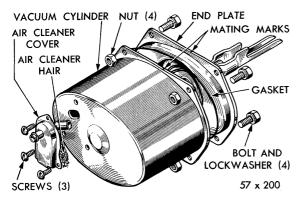
Fig. 23 — Removal of Air Cleaner and Vacuum Cylinder)
