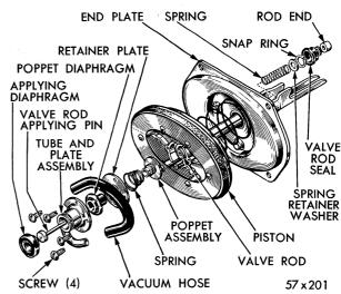
Fig. 24 — Disassembly of Tube and Plate Assembly
