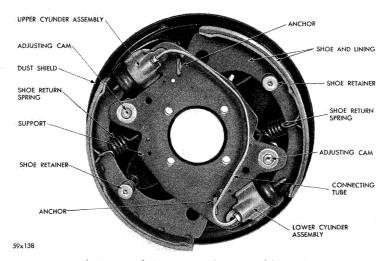
Fig. 19 — Total Contact Brake Assembly (Front)
