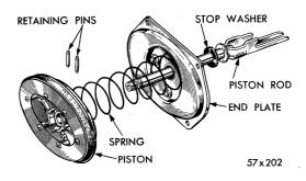
Fig. 25 — Removal of Vacuum Piston, Spring and Piston Rod
