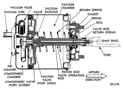
Fig. 21 — Power Brake Unit (Sectional View)
