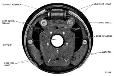
Fig. 20 — Total Contact Brake Assembly (Rear)
