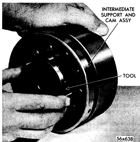
Fig. 82—Installation of Tool C-3527 in Intermediate Support and Cam Assembly
