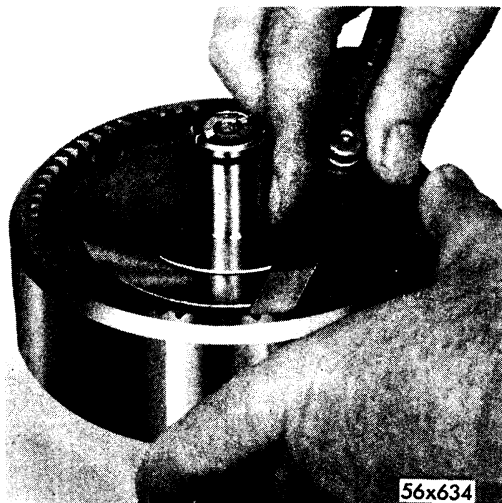
Fig. 78—Checking Clearance Between Kickdown Annulus Gear Snap Ring and Intermediate Shaft Assembly
