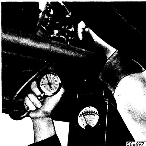
Fig. 23—Checking Line Pressure
