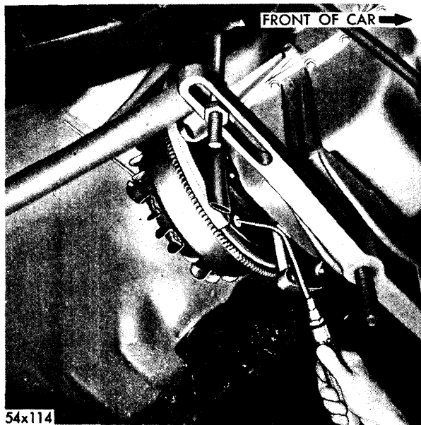
Fig. 118—Heating Torque Converter (Housing Removed to Show Heating Operation)
