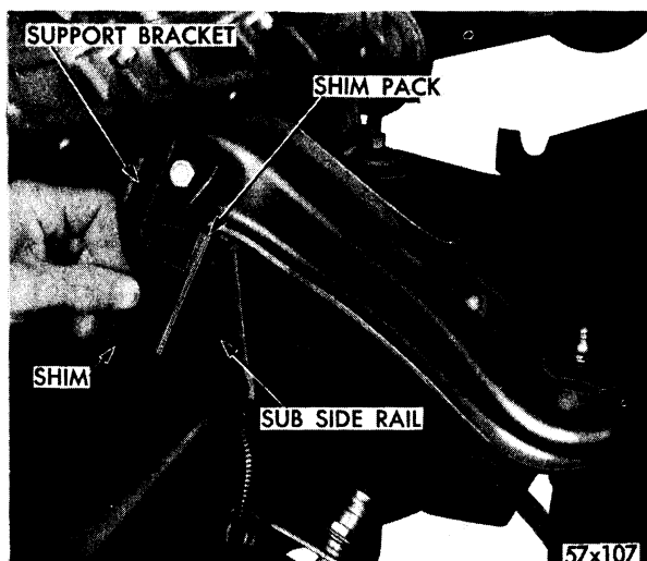
Fig. 25—Removing Shims to Adjust Camber or Caster
