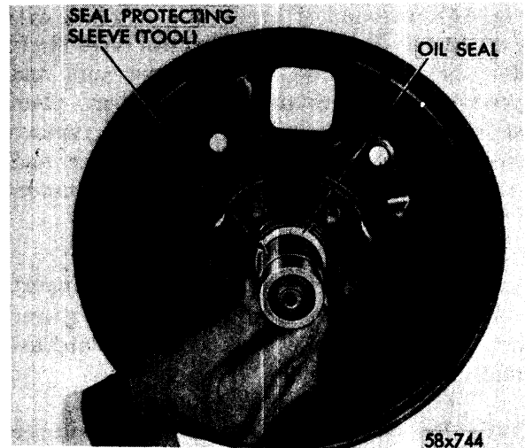
Fig. 15—Removing or Installing Rear Brake Support Shield with (Tool C-745)
