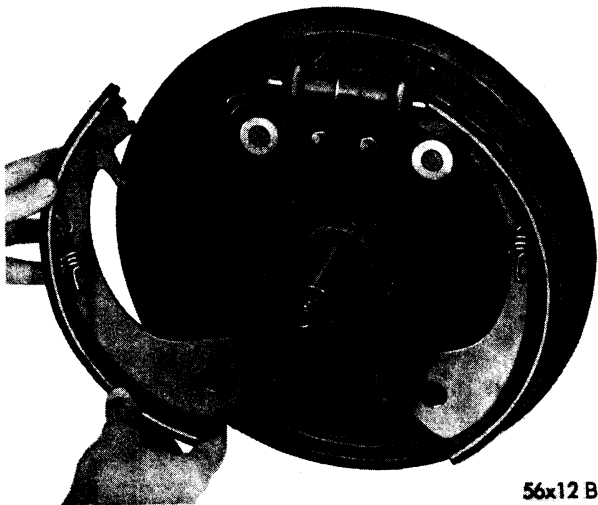
Fig. 13—Removing or Installing Rear Brake Shoe
