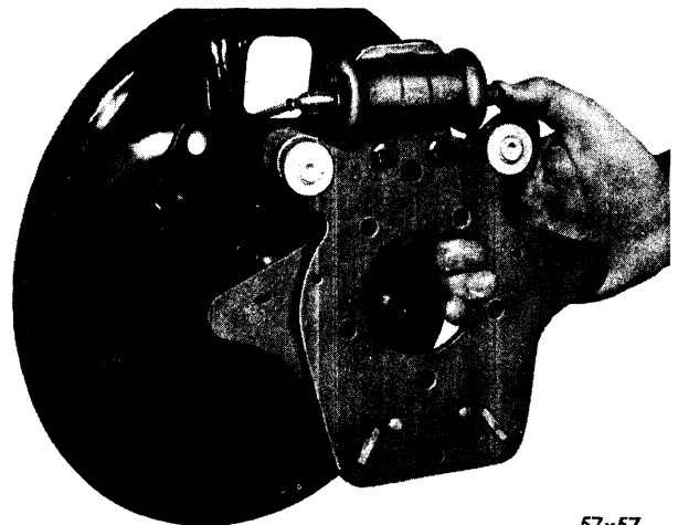
Fig. 16—Installing Rear Brake Support Plate
