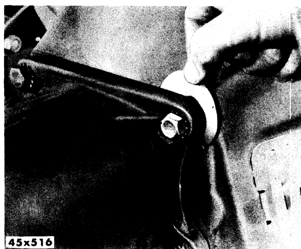
Fig. 11—Inserting Shim Between Transmission and Clutch Housing
