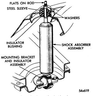
Fig. 12—Front Shock Absorber
