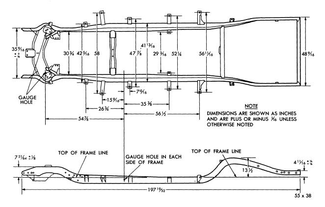
Fig. 2 – Frame Dimensions (Custom Imperial)
