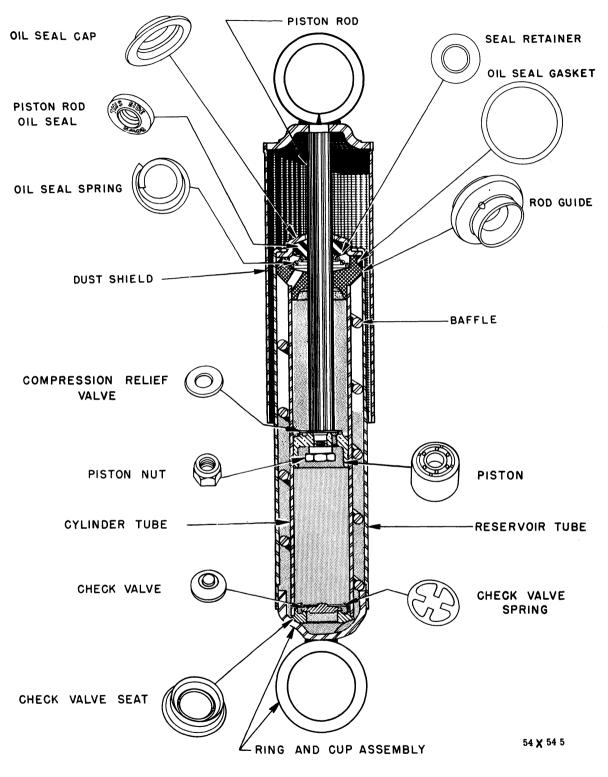
Fig. 13—Rear Shock Absorber (Sectional View)
