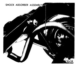
Fig. 15-Rear Shock Absorber Installed
