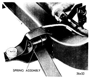
Fig. 5—Rear Spring Front Mounting
