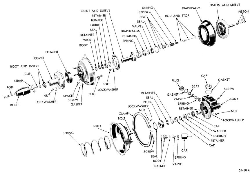
Fig. 70—Power Brake (Disassembled View) (Late Design)
