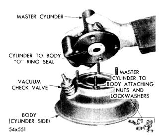
Fig. 74—Removing or Installing Hydraulic Cylinder
