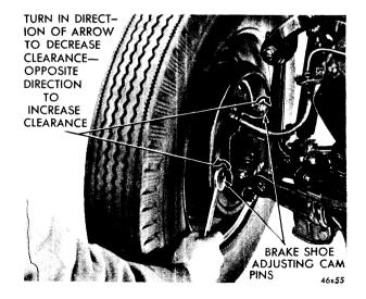
Fig. 11—Turning Brake Adjusting Cam (Typical View)
