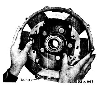
Fig. 49—Removal and Installation of Pressure Plate Assembly (Front Disc Brake)
