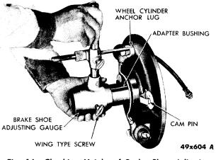
Fig. 16—Checking Height of Brake Shoe Adjusting Pin, Using Tool MT-19-L
