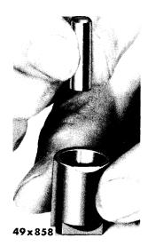
Fig. 57—Inserting Dummy Shaft in Adjuster Sleeve
