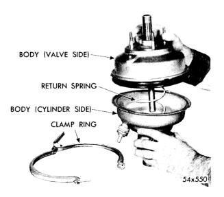
Fig. 73—Removing Power Piston and Guide
