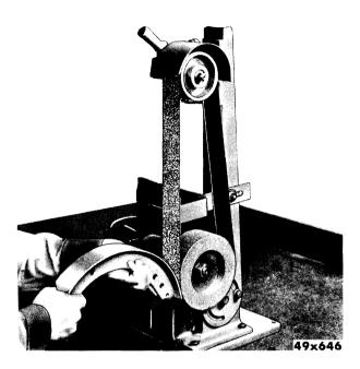
Fig. 29-Sanding Brake Shoe
