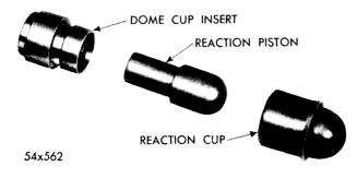
Fig. 85—Reaction Piston Insert and Dome Cup
