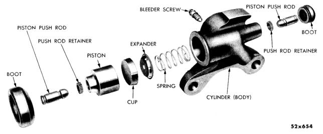
Fig. 40—Front Wheel Brake Cylinder (Disassembled View)
