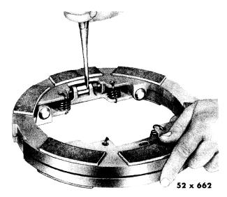
Fig. 50—Releasing Automatic Adjuster (Front or Rear Pressure Plate)
