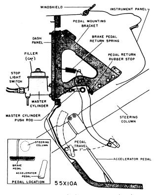
Fig. 3—Master Cylinder Location and Linkage
