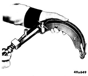
Fig. 33—Tightening Wing Nut Against Pressure Spring
