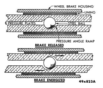
Fig. 39—Self-Energization Illustrated
