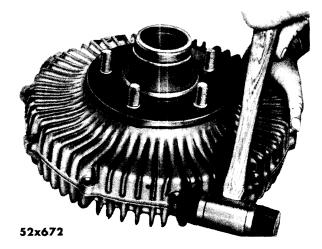
Fig. 48—Separating Inner and Outer Housings (Front Disc Brake)
