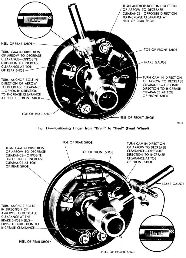
Fig. 18—Positioning Finger from "Drum" to "Heel" (Rear Wheel)
