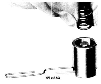
Fig. 62—Positioning Adjuster Spring in Sleeve
