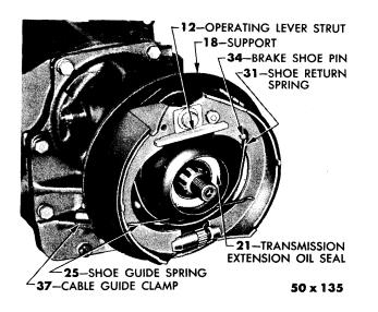
Fig. 25—Internal Expanding Hand Brake
