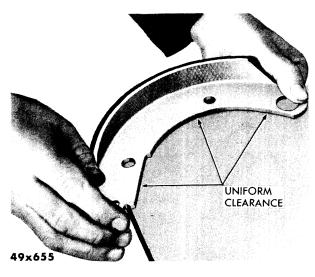
Fig. 15—Checking Shoe for Twist
