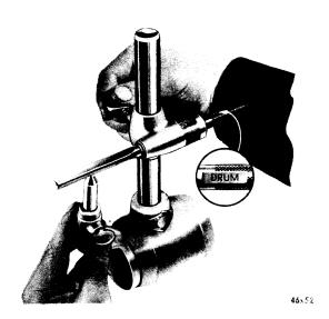
Fig. 20—Setting Brake Shoe Gauge
