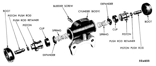
Fig. 41—Rear Wheel Brake Cylinder (Disassembled View)
