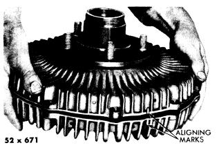
Fig. 47—Brake Housing Aligning Marks (Front Disc Brake)
