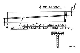
Fig. 92-Grooved Brake Lining
