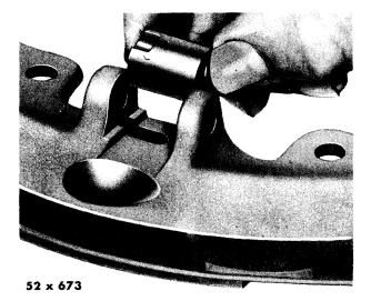
Fig. 64—Positioning Sleeve on Pressure Plate
