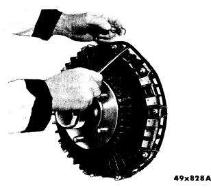
Fig. 45—Removal and Installation of Dampener Springs and Clips (Front Disc Brake)
