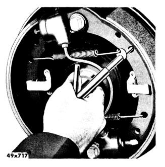
Fig. 5—Removing and Installing Brake Shoe Return Spring
