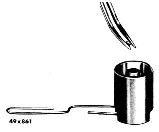
Fig. 60-Installing Adjuster Balls in Sleeve
