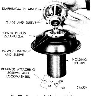
Fig. 77—Removing Guide Assembly from Power Piston Assembly
