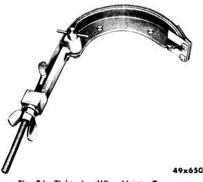
Fig. 34—Tightening Wing Nut to Compress Pressure Spring
