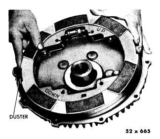
Fig. 54—Removing or Installing Pressure Plate Assembly (Rear Disc Brake)
