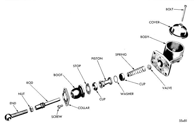
Fig. 4—Master Cylinder (Disassembled View)
