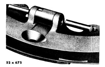
Fig. 66—Forcing Dummy Shaft Out of Adjuster Sleeve
