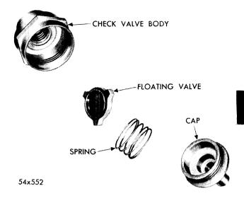
Fig. 75—Check Valve (Disassembled View)
