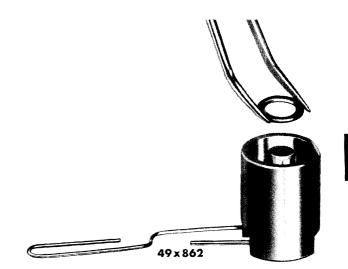
Fig. 61—Installing Adjuster Washer in Sleeve
