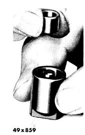
Fig. 58—Positioning Adjuster Bushing Over **Dummy Shaft**
