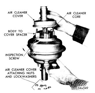
Fig. 72-Removing or Installing Air Cleaner Cover
