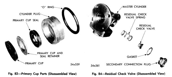
connection plug, and residual check valve seat. Lift out residual check valve assembly, and residual check valve spring. Discard residual check valve assembly and seat. (Refer to Fig. 84.)
