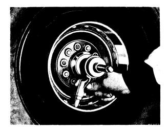
Fig. 19—Checking Brake Drum Diameter
