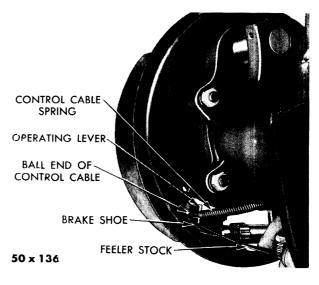
Fig. 28—Clearance Between Lever and Brake Shoe Table
