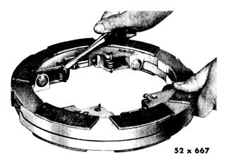
Fig. 55—Removal or Installation of Pressure Plate Retaining Springs (Front or Rear Disc Brake)
