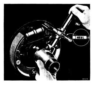
Fig. 21—Checking Toe Adjustment
