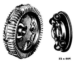
Fig. 53—Removing or Installing Rear Disc Brake Hub and Housing
