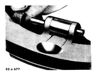
Fig. 68—Installing Lubricating Washer on Adjuster Rod
