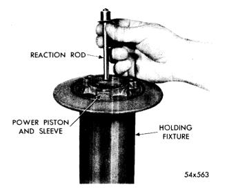
Fig. 86—Installing Reaction Rod
