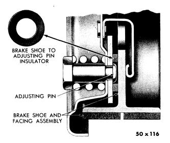
Fig. 91—Insulating Washer Installed
