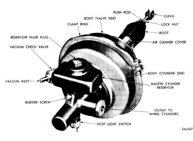
Fig. 69—Power Brake Unit
