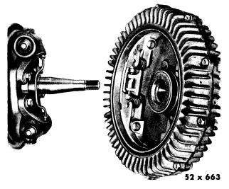
Fig. 44—Removing or Installing Hub and Brake Housing Assembly (Front Disc Brake)
