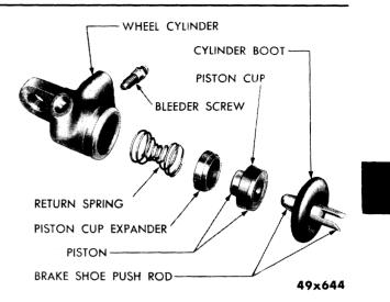
Fig. 7—Front Wheel Cylinder (Disassembled View)
