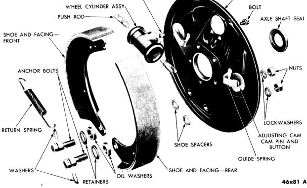
Fig. 2-Rear Brake (Disassembled View)
