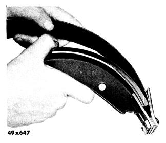
Fig. 31—Installing Shoe and Lining in Clamp
