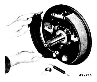
Fig. 6—Removing Brake Shoe
