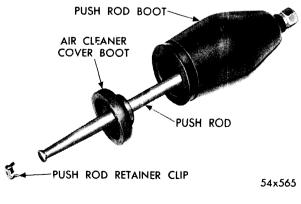
Fig. 88—Push Rod (Disassembled View)
