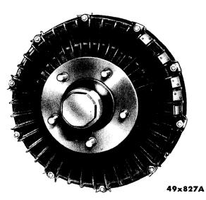
Fig. 43-Front Disc Brake
