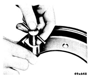
Fig. 32—Inserting Clamp Pin Anchor Hole
