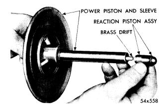
Fig. 81-Removing Reaction Piston Assembly
