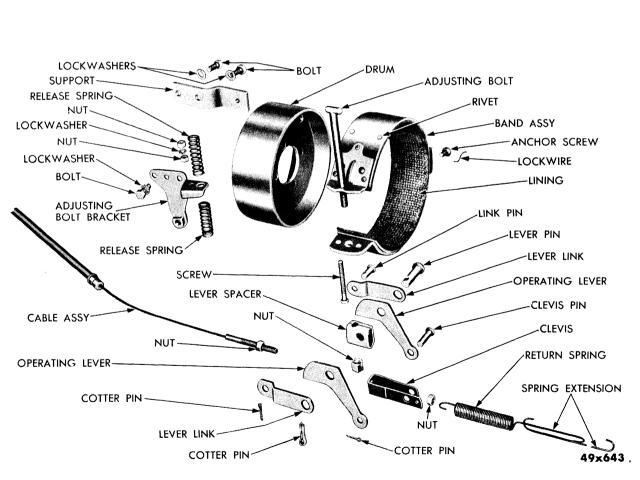
Fig. 23—Hand Brake (Disassembled View—External Type)
