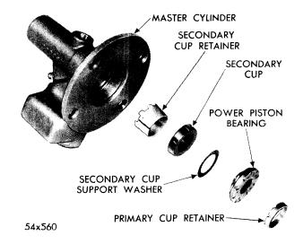
Fig. 83—Secondary Cup Parts (Disassembled View)
