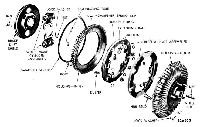
Fig. 37—Rear Disc Brake (Disassembled View)
