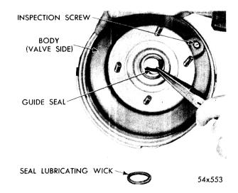
Fig. 76—Removing Guide Seal and Lubricating Wick
