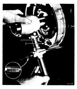
Fig. 22—Checking Heel Adjustment (Items 1 and 2 are Anchor Bolts)
