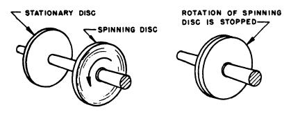
Fig. 38—Relation of Spinning and Stationary Discs
