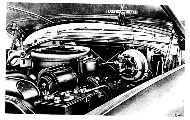
Fig. 90—Brake Power Unit Installed
