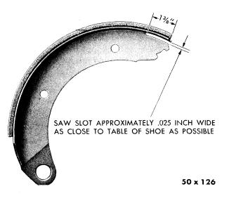
Fig. 93-Slot in Web of Shoe
