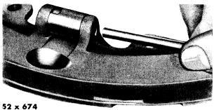
Fig. 65—Inserting Adjuster Rod Into Pressure Plate
