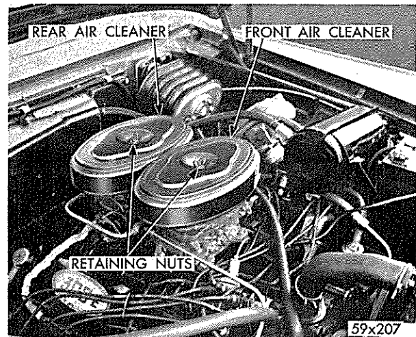
Fig. 6 - Carburetor Air Cleaners Installed
