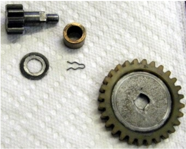
Gears and bushing shown with other pieces. Small clip in center was used in assembly. Large gear shown is replacement for broken unit.
