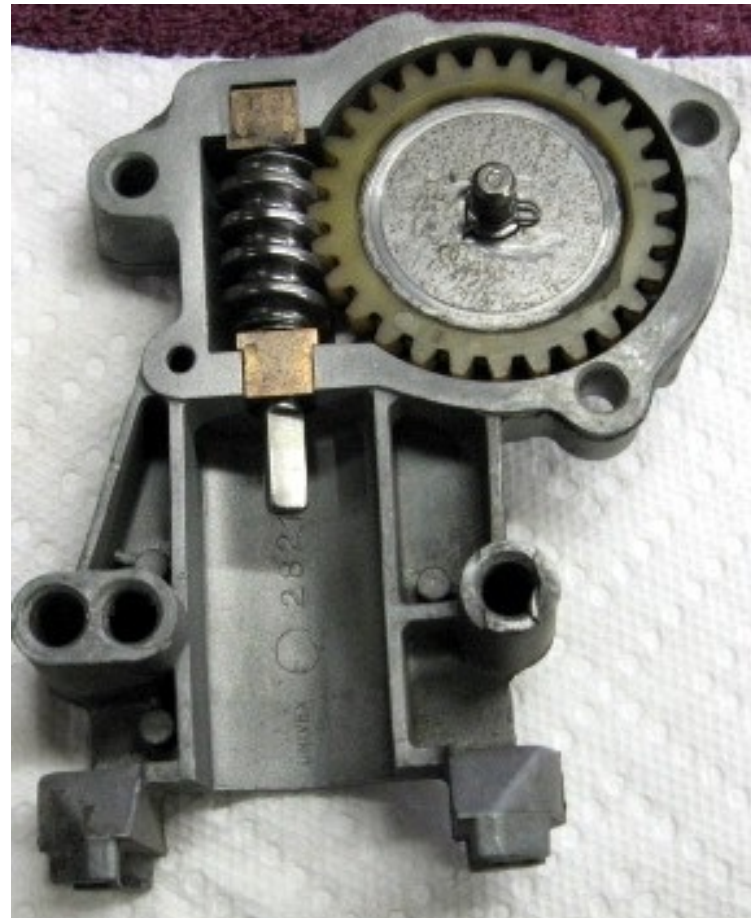
Reassembled unit shows spring clip on shaft and is ready to operate.
