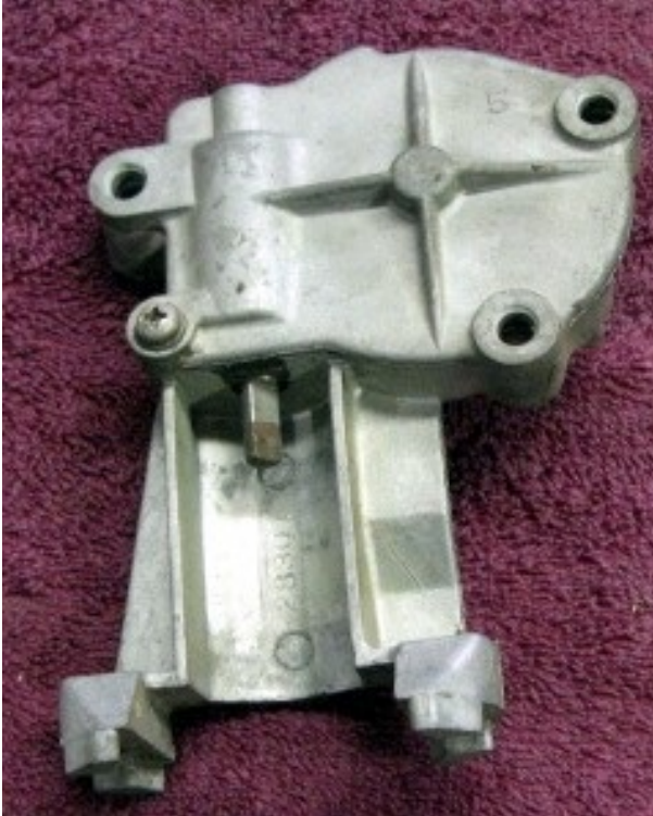
Chrysler Power Window Gear Drive used from 60 through 64. This one has a broken gear.
