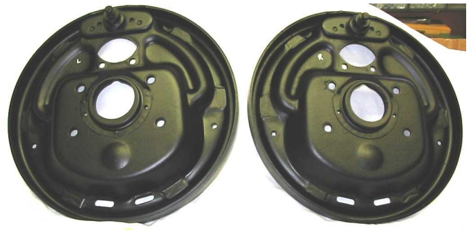
Freshly painted backing plates
