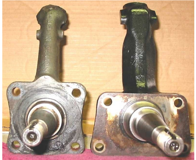
Old spindle on left, replacement on right. 64 spindle is huskier and upper portion is more recessed to accommodate recessed backing plate for 3" brakes.
